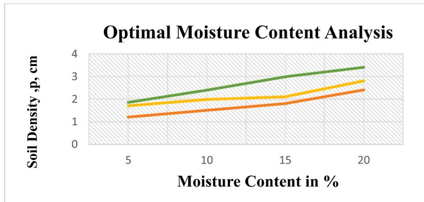
Fig. 4. Optimal moisture content analysis.
